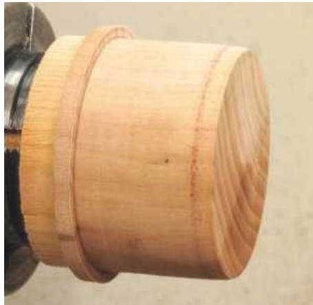
STEP 20. The fit does need to be really tight here so remember to creep up on the correct diameter rather than going for it hell for leather. Remember that it's much easier to take more off than trying to add it back on
